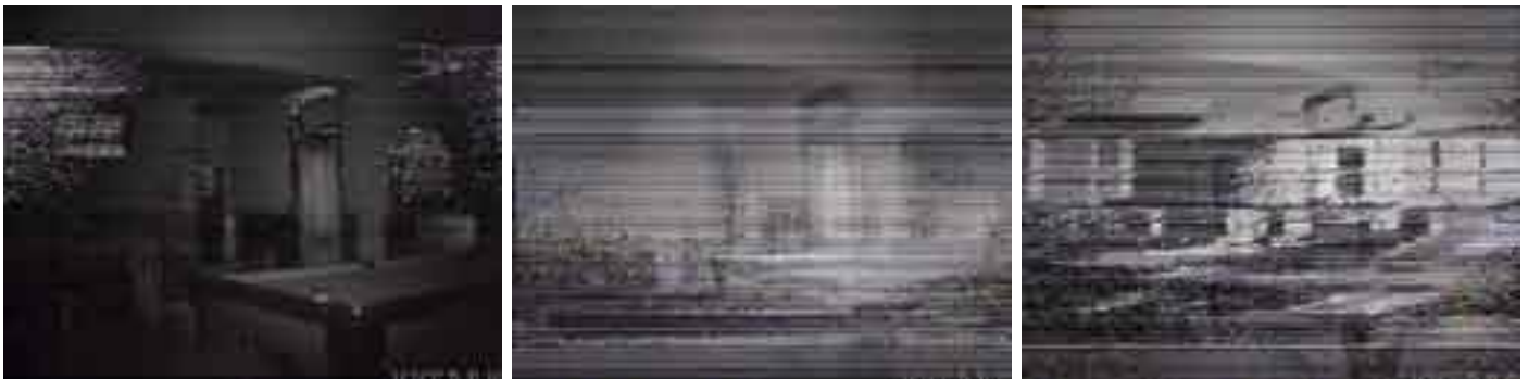
Interference noted on the DVR camera 4 in the pool room over a period of about 1 1/2 minutes.
